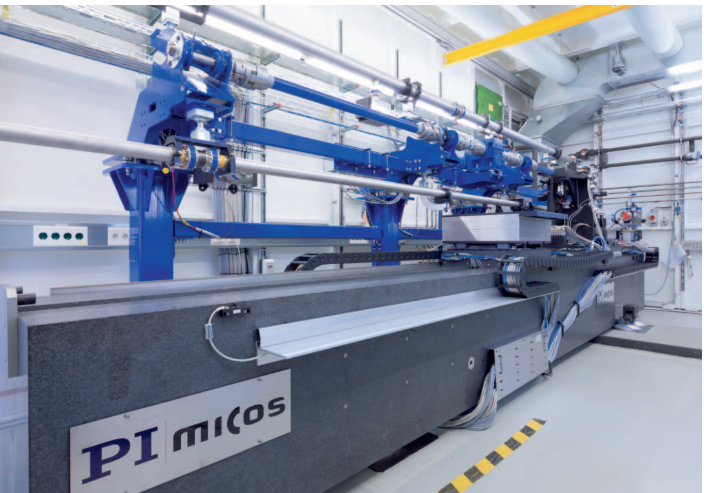
Experimental setup of nanotomography at the P05 beamline, PETRA III, DESY research center (German Electron Synchrotron) in Hamburg, Germany (Image: PI / HZG)
